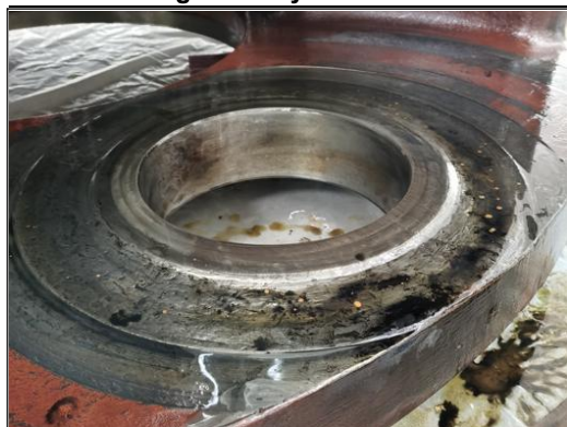
200 Planetary Carrier - Wear at the end of the 251 bearing position, needs machining and adding a locking pin
