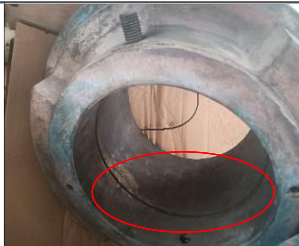
150 Bearing - Wear, scratches
