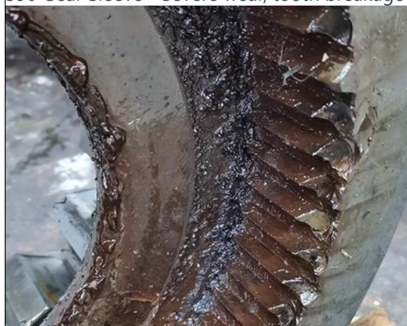
390 Gear Sleeve - Severe wear, tooth breakage
