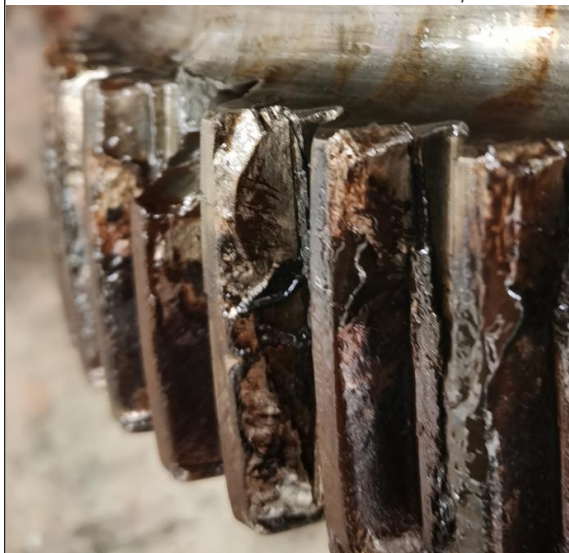
400 Intermediate Shaft - Severe wear, tooth breakage
