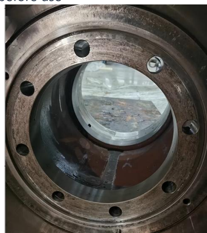
125 Spacer Ring - End surface wear, needs repair before use
