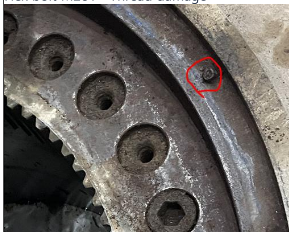
Internal inspection of the 451 bearing hole in the gearbox is intact. After PT testing, no cracks were found in the internal gear ring of the gearbox, continue use.
