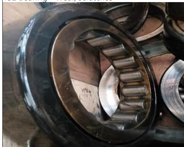
152 Bearing - Wear, scratches
