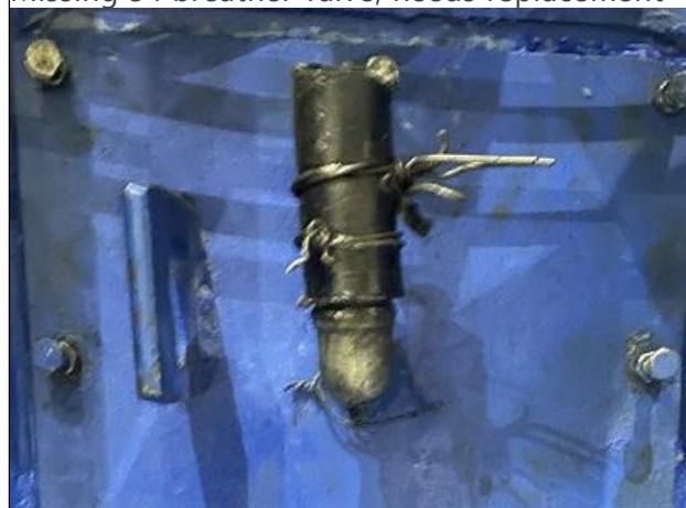
Missing 54 breather valve, needs replacement
