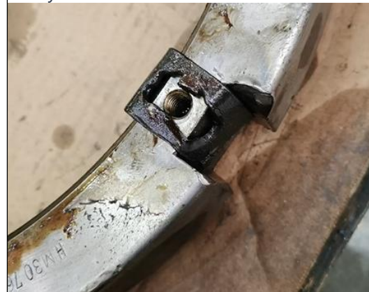
200 Planetary Carrier - Wear on the upper pin hole, out-of-roundness
