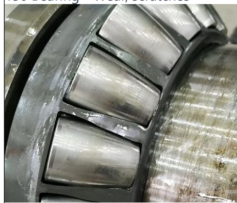
152 Bearing - Wear, scratches
