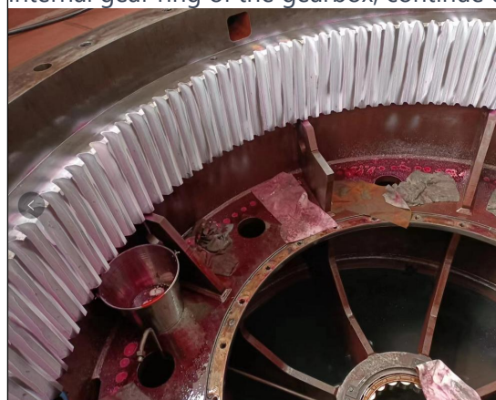
Internal inspection of the 451 bearing hole in the gearbox is intact. After PT testing, no cracks were found in the internal gear ring of the gearbox, continue use.
