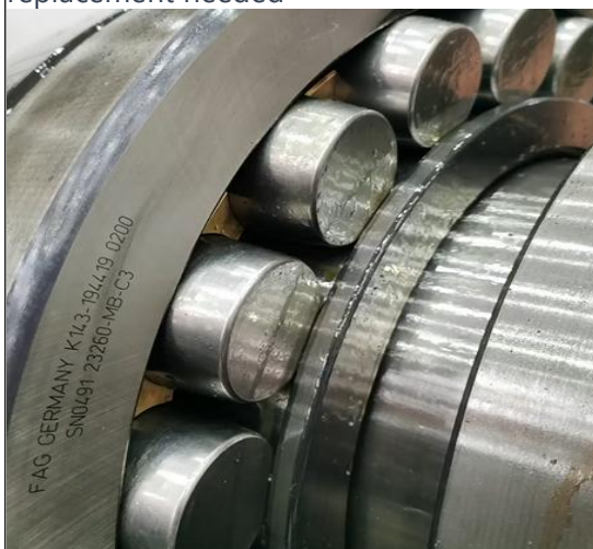
251 Bearing - Obvious scratches on rolling elements
