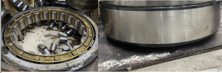
451 Bearing - Scratches, foreign object entry
