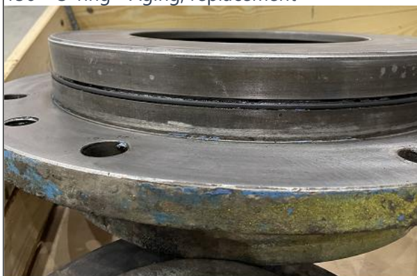
151 Bearing - Foreign object entry, needs dismantling, replacement needed
