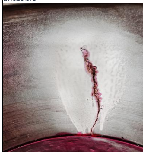
314 Planetary Wheel Bearing Adjustment Ring - Wear, needs remanufacturing
