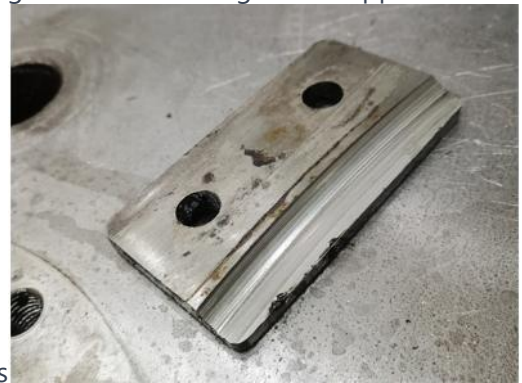
411 Lock Nut Stop Piece - Deformed, needs to be newly made
