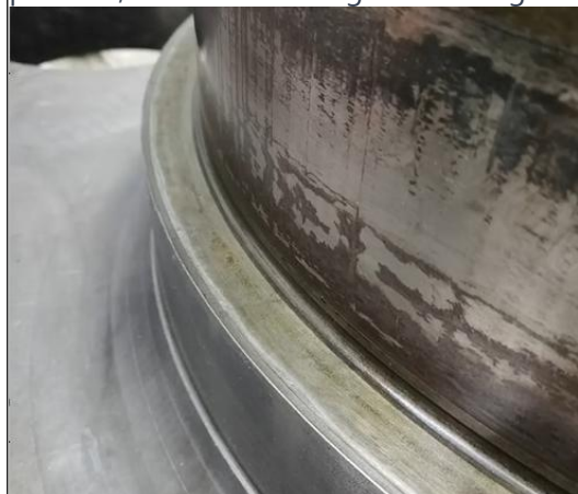
Planetary Wheel Tooth Surface - Normal wear
